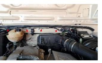
compartment. Apply a little washing-up liquid to the beginning of the wiring harness so that it can slide easily through the rubber. Grasp the cable tie on the engine compartment side and carefully pull the wiring harness through until it is long enough to connect it to the control unit.
