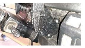
longer required as the flap is then always open and has therefore become superfluous. The upper screw is located directly behind a part of the dashboard, which must either be partially dismantled for good accessibility, or you can leave this screw in the hole after unscrewing it and secure it with a nut.
